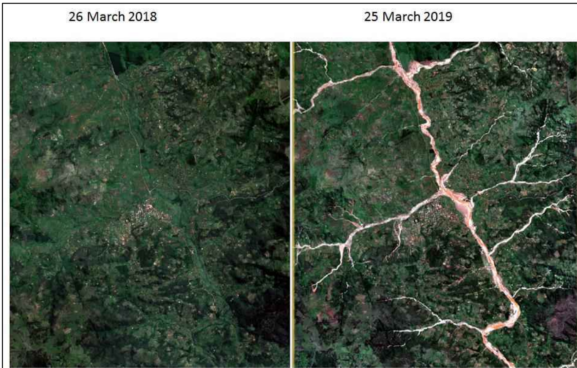
Figure 8.3 Landslides and widening of the Nyahode River 13 km south of Chimanimani due to rainfall and floods during the Cyclone Idai period (Source: Sentinel 2 images from the European Space Agency).
